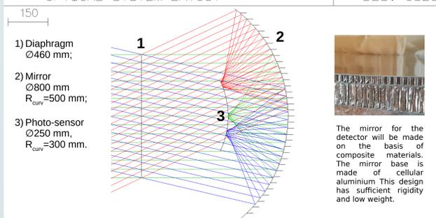
The mirror for the detector will be made on the basis of composite materials. The mirror base is made of cellular aluminium. This design has sufficient rigidity and low weight.
