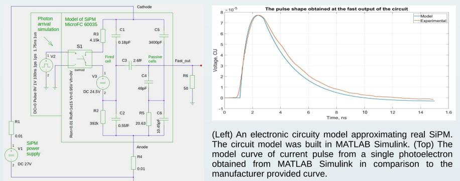
(Left) An electronic circuit model approximating real SiPM. The circuit model was built in MATLAB Simulink. (Top) The model curve of current pulse from a single photoelectron obtained from MATLAB Simulink in comparison to the manufacturer provided curve.
