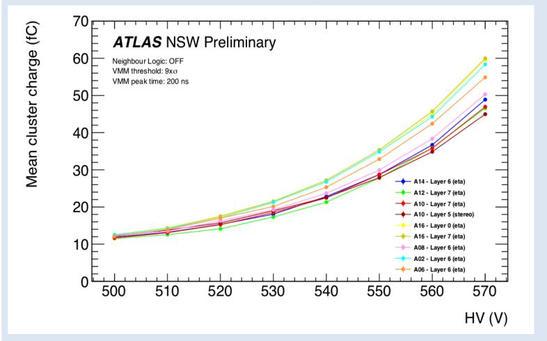
Mean cluster charge vs amplification voltage
