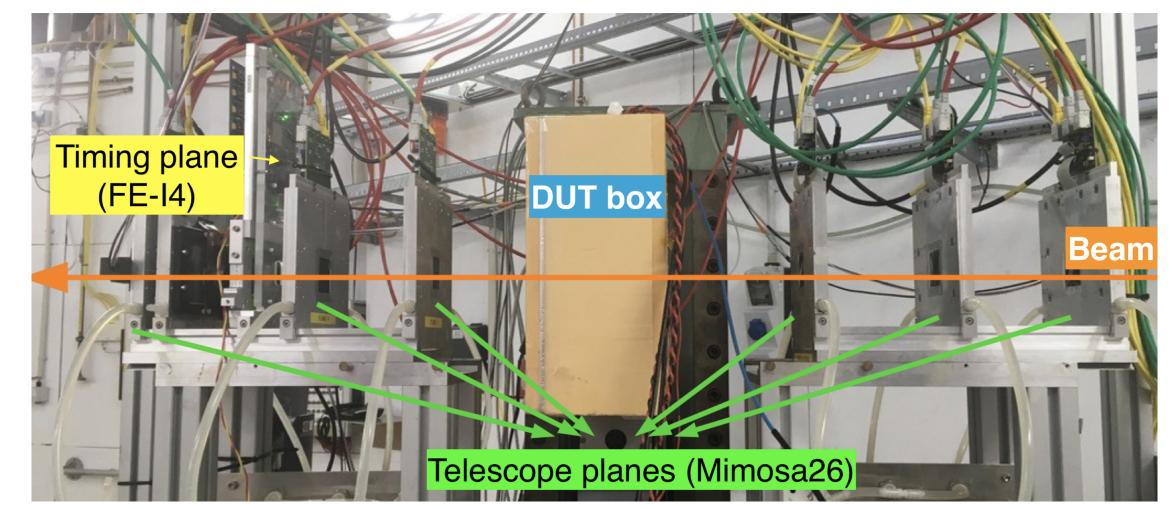
• A timing-plane (FE-I4), to compensate the large time integration of the pixel planes (~ 115  $\mu$ s) with respect to the DUT (~  $25 \,\mu s$ ) through precise measurement of the particle arrival time.
