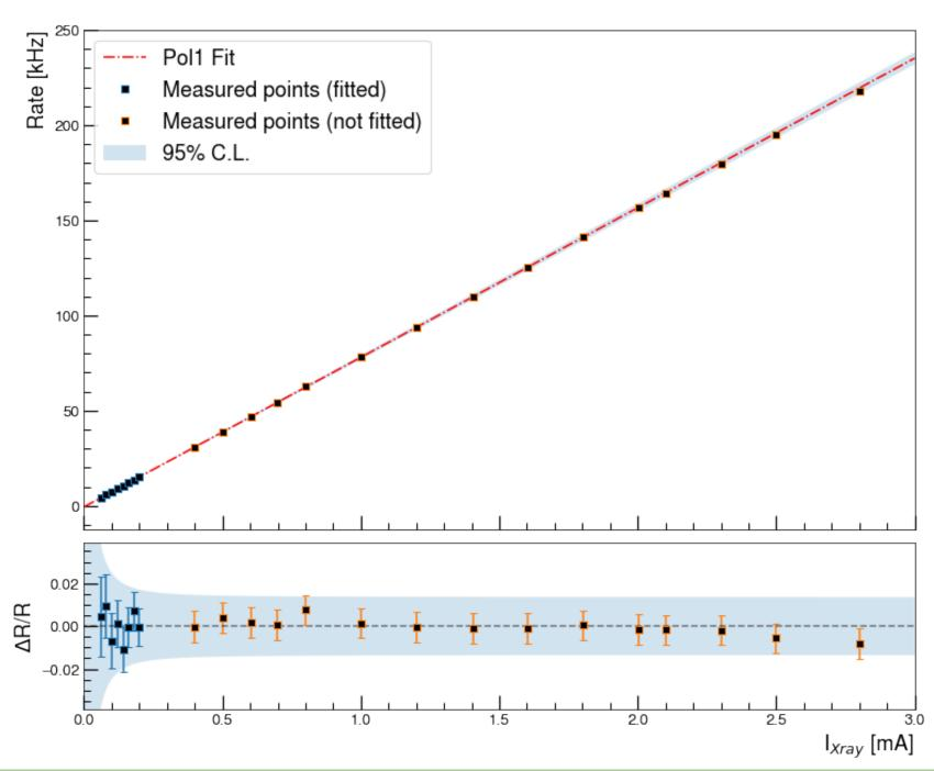
With X-Ray gun rates are directly measured for low intensities, and then are extrapolated for high rates.
