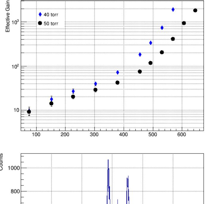
THGEM effective gain as function of voltage in low-pressure TPC in isobutane at pressures of 40 torr and 50 torr
