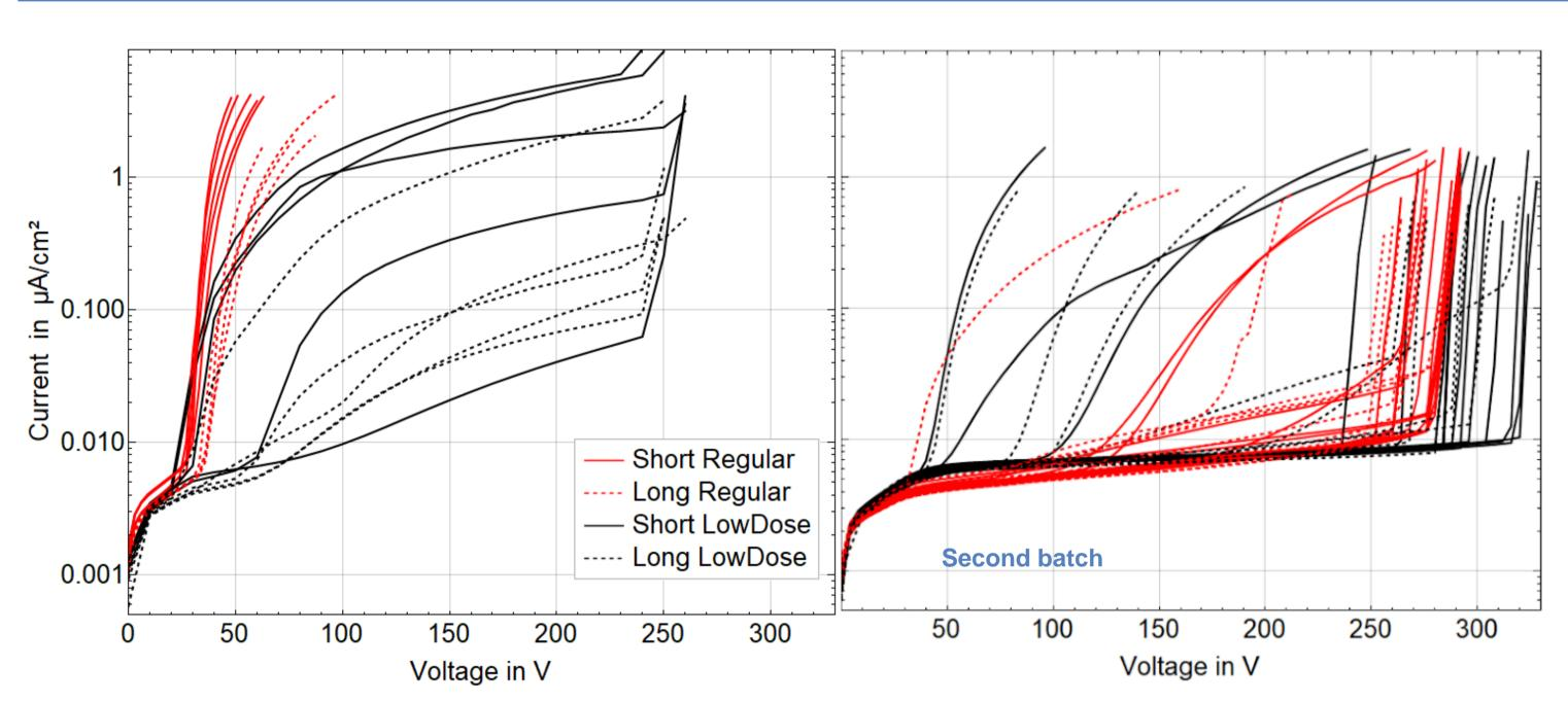
First batch: low concentration backside implant and not metallization Second batch: higher concentration backside implant and metallization
