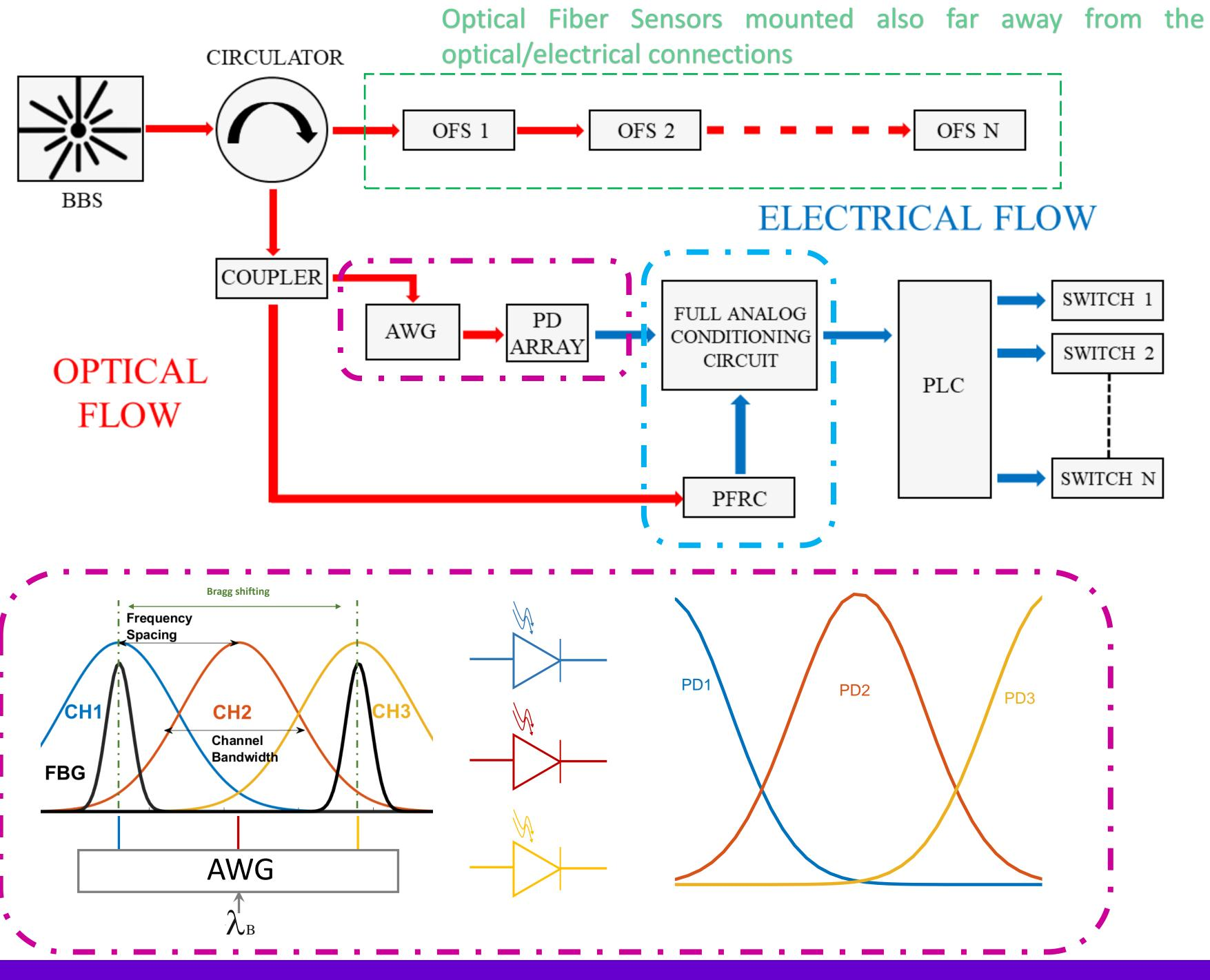
To take advantage of the FOS sensing feature within a safety monitoring system to be used in harsh environments (like DSS frontend) an optoelectronic interrogation system must be:
