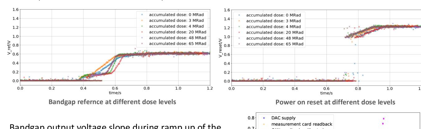
Bandgap output voltage slope during ramp up of the power supply is different for different levels of the accumulated dose. The slope is less steep due to the fact ≥ 0.5 that radiation dose rate is much slower. Because of this threshold of the NMOS transistor changes for this particular CMOS process.
