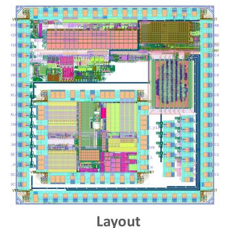
Complete digital logic of the MOPS chip has been implemented using Triple Modular Redundancy (TMR) to mitigate SEUs effects
