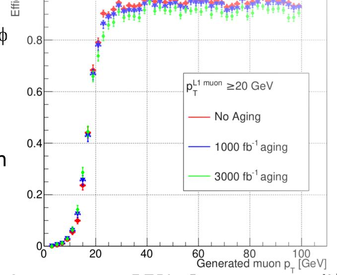
Overall efficiency over 95% for muons with p<sub>T</sub> > 20 GeV, with a turn on width of ~5 GeV. Estimated to be the MTF most affected by ageing effects, due to its dependence on the outermost DT:
