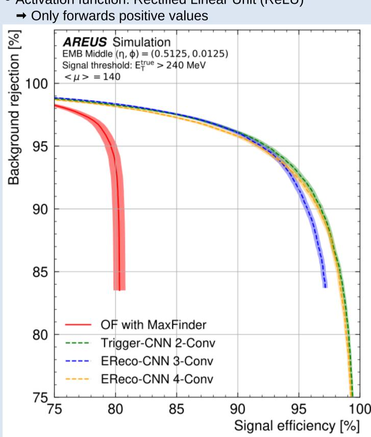
→ Increased signal efficiency and background rejection compared to OF for trigger as well as combined network
