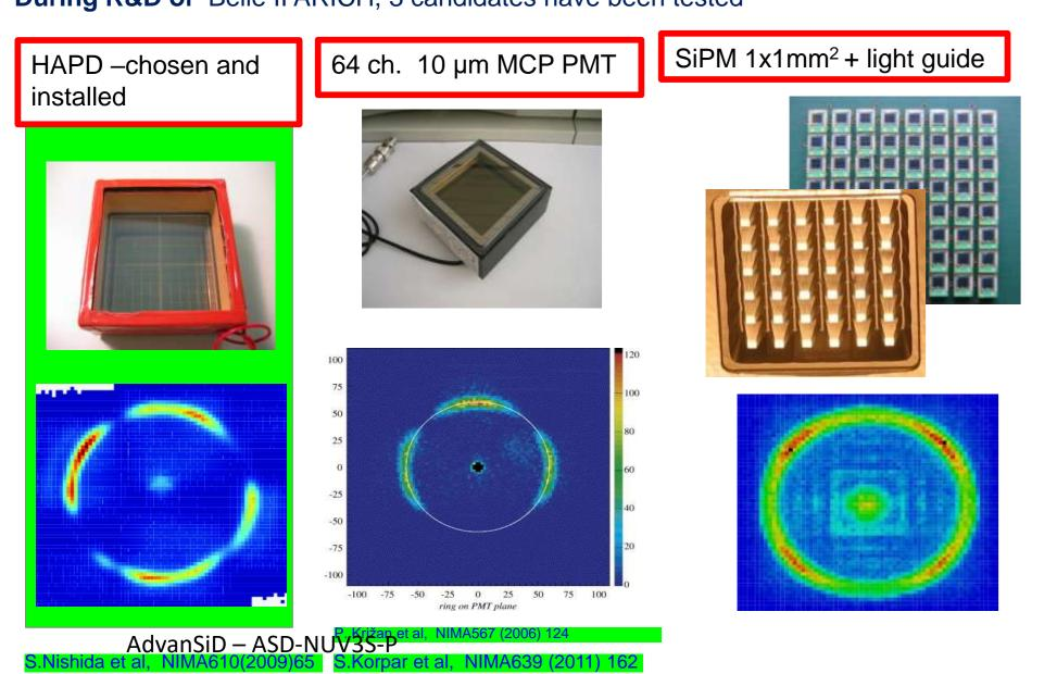
This work focuses on the use of silicon photomultipliers as a photon detector.
