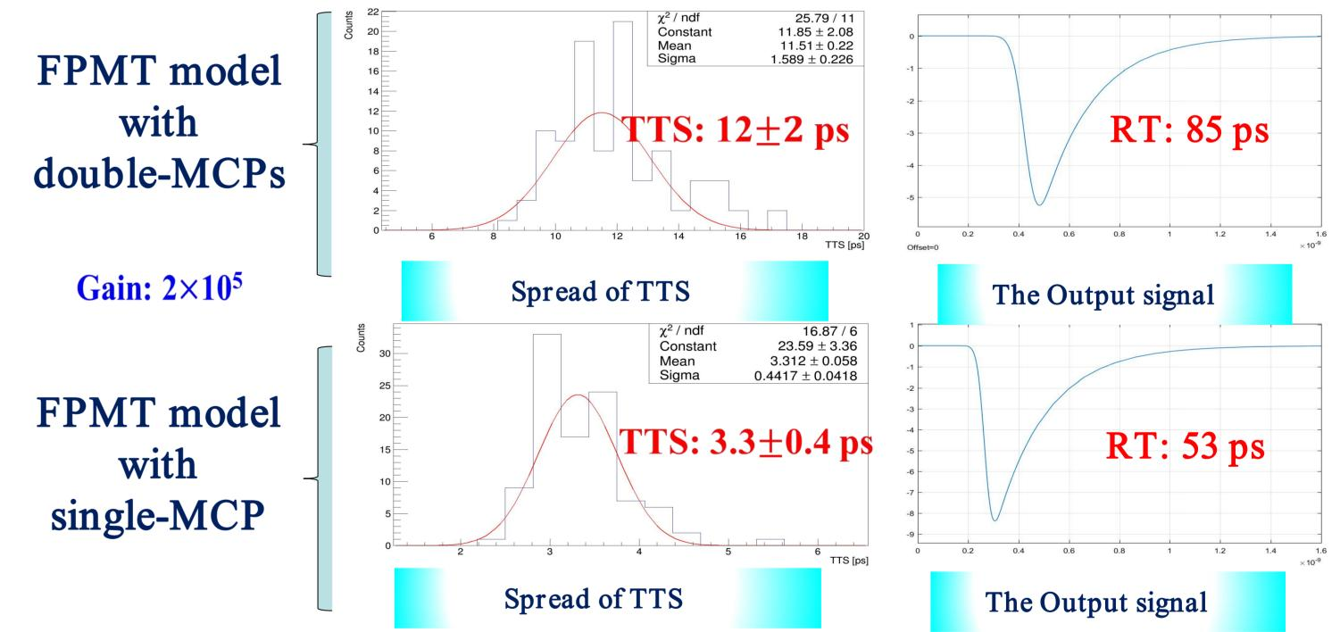
> Through multiple simulations, the spread of TTS is obtained and the output signal is obtained by using a equivalent circuit.
