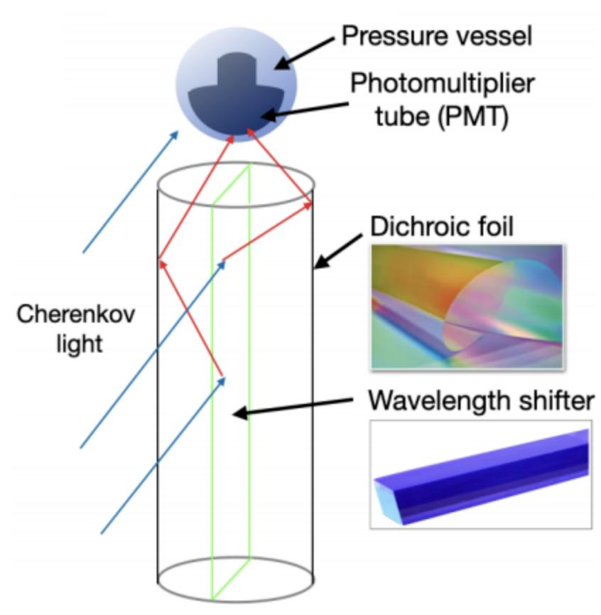
Thin dichroic foil is wrapped in cylinder shape, which is deformable (does not resist pressure from freezing water)
