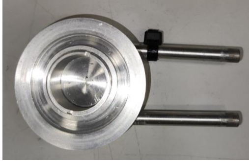
Metallic Li for higher production \rightarrow cooled target
