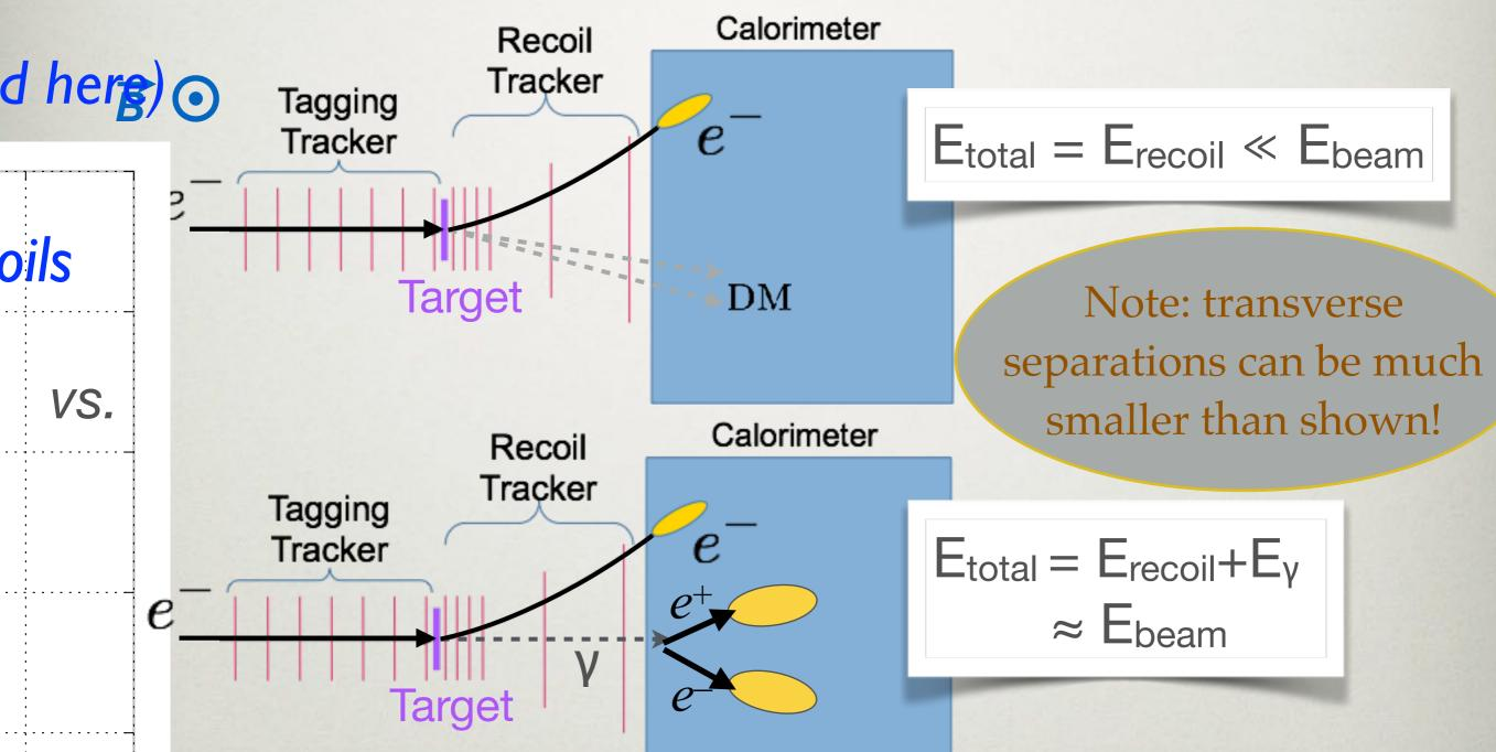
Trigger on low energy deposition  $\rightarrow \sim 400$  Hz of DM-like events from  $\sim 25$  MHz of bunches.
