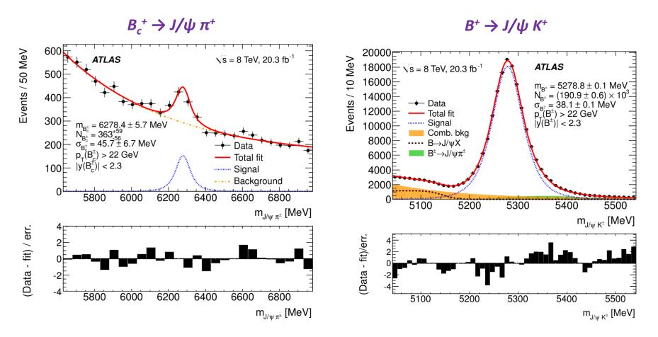
$B_c^+$  and  $B^+$  yields measured using di-muon trigger
