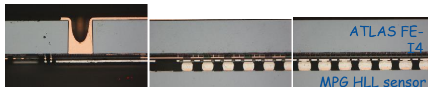
Cross section of module with 80µm thick ATLAS FE-I4 backside TSV ROC
