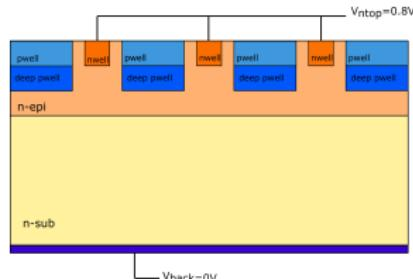
►  $V_{top} = 0.8V$ , starts depletion from back side
