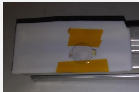
Calibration sample (Zr, K, Br, Zn, Mn, Ti)
