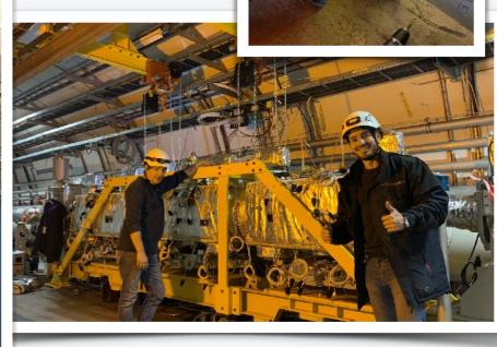
Beam Wire Scanner and Beam Gas Curtain
