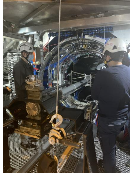
Handling test of the ITS chassis to simulate the installation of the Top and bottom ITS Half barrels inside the Cage
