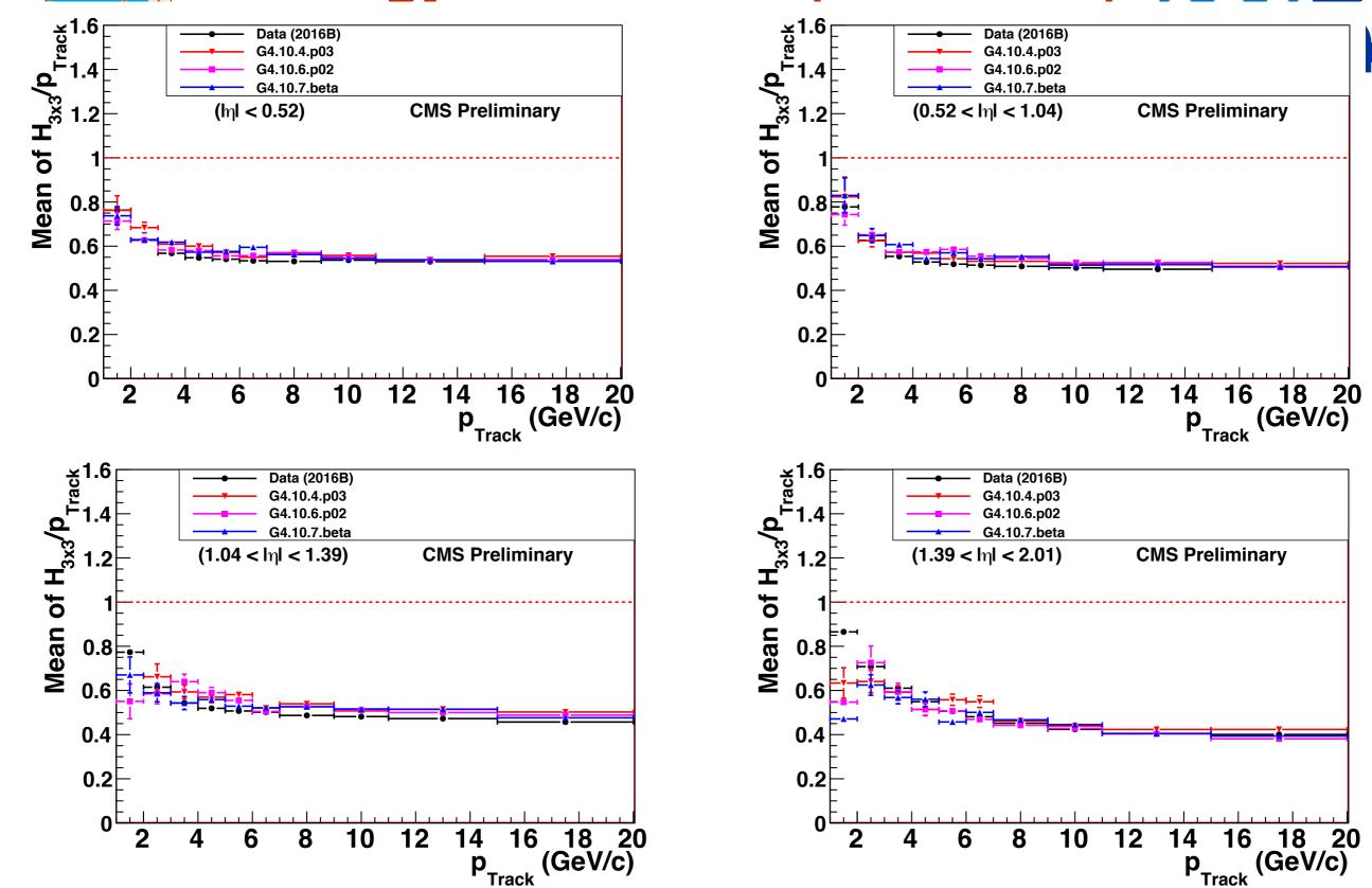
Mean of the ratio of energy measured in a 3x3 matrix in the HCAL to track momentum in 4 regions of the detector: central barrel (top left); side barrel (top right); transition region (bottom left); endcap (bottom right)
