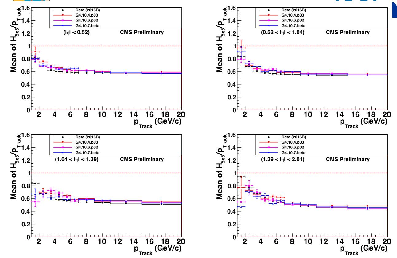
Mean of the ratio of energy measured in a 5x5 matrix of the HCAL to track momentum in 4 regions of the detector: central barrel (top left); side barrel (top right); transition region (bottom left); endcap (bottom right)
