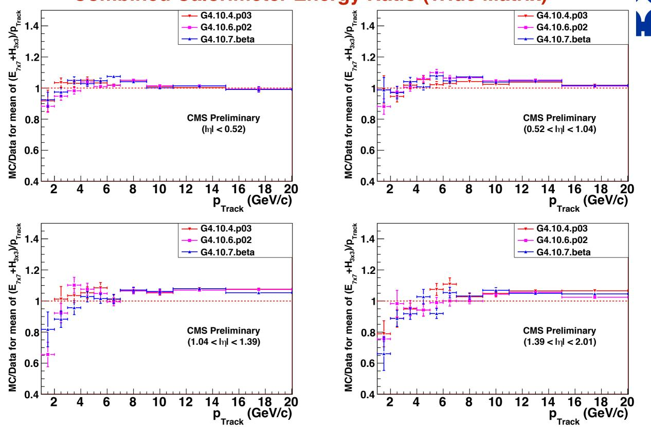
Ratio of the mean energy response in a wide matrix of ECAL and HCAL between MC and data for four regions of the calorimeter: central barrel (top left); side barrel (top right); transition region (bottom left); endcap (bottom right) 19 **Geant4 Technical Forum** S. Banerjee, V. Ivantchenko
