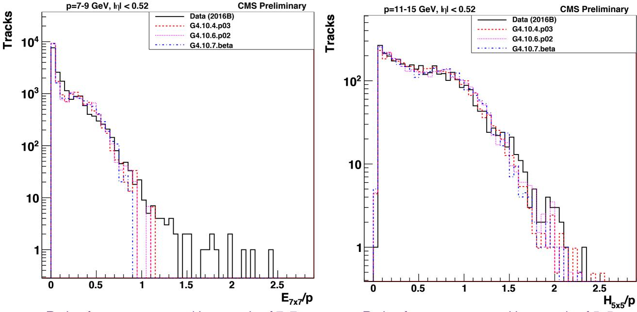
Ratio of energy measured in a matrix of 7x7Ratio of energy measured in a matrix of 5x5crystals around the hit point in the barreltowers around the hit point in the endcap hadronelectromagnetic calorimeter for tracks ofcalorimeter for tracks of momentum between 11momentum between 7 and 9 GeV.and 15 GeV.
