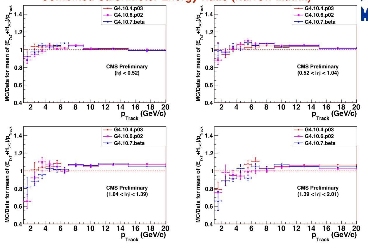
Ratio of the mean energy response in a narrow matrix of ECAL and HCAL between MC and data for four regions of the calorimeter: central barrel (top left); side barrel (top right); transition region (bottom left); endcap (bottom right) 18 **Geant4 Technical Forum** S. Banerjee, V. Ivantchenko
