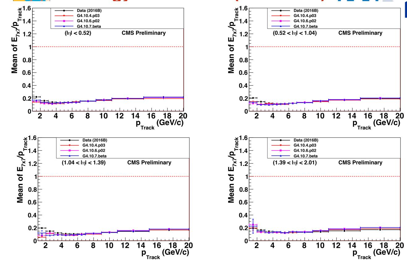
Mean of the ratio of energy measured in a 7x7 matrix in the ECAL to track momentum in 4 regions of the detector: central barrel (top left); side barrel (top right); transition region (bottom left); endcap (bottom right)
