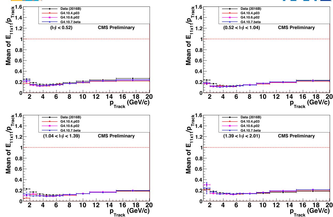
Mean of the ratio of energy measured in a 11x11 matrix in the ECAL to track momentum in 4 regions of the detector: central barrel ((top left); side barrel (top right); transition region (bottom left); endcap (bottom right)
