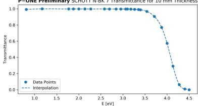
P-ONE Preliminary SCHOTT N-BK 7 Transmittance for 10 mm Thickness
