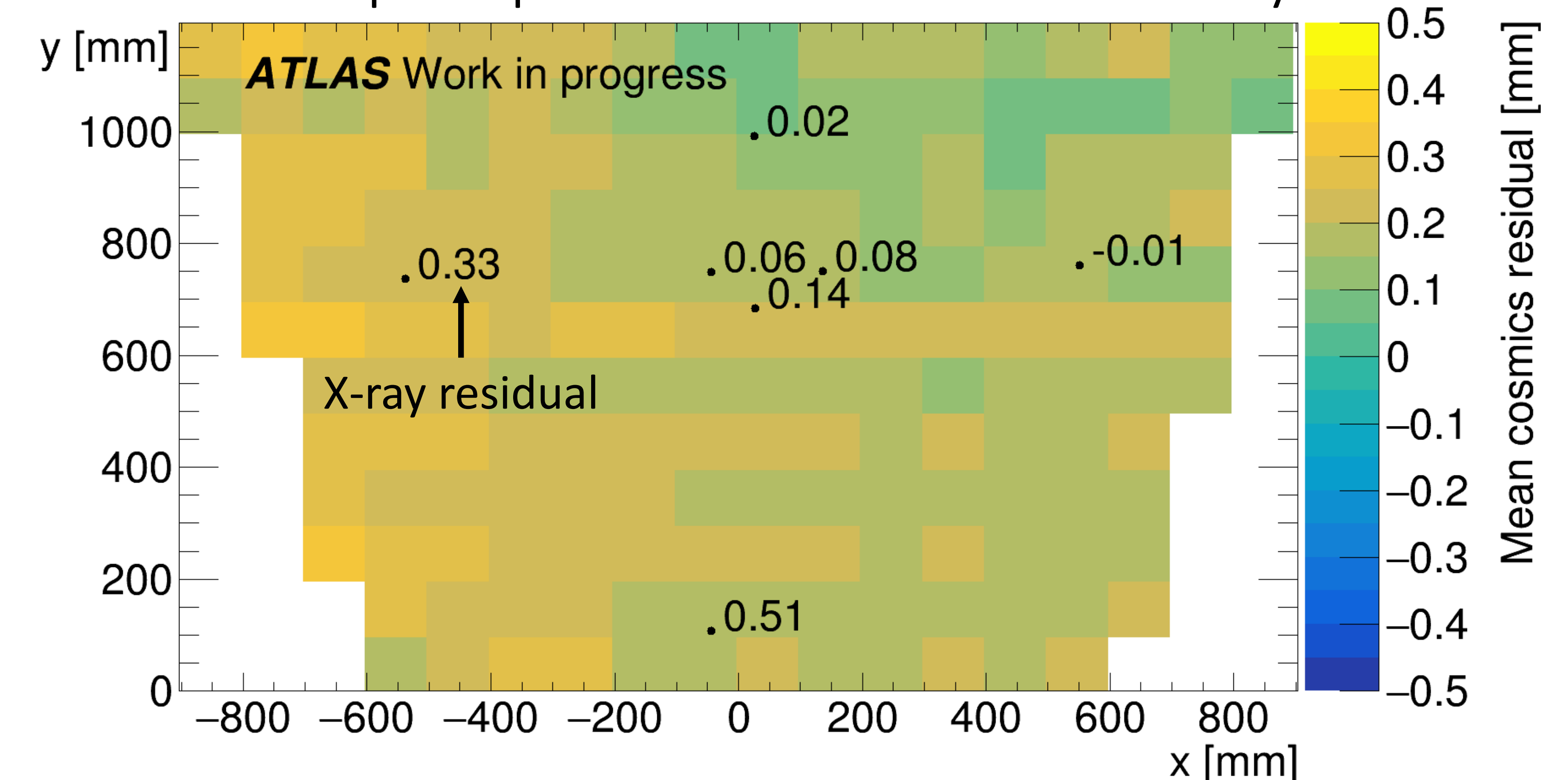
Fig. 3 Mean cosmic residuals on layer 2 w.r.t layers 1 and 4 for quadruplet QL2.C.4. The x-ray residuals (in mm) are represented by the annotated black points.
