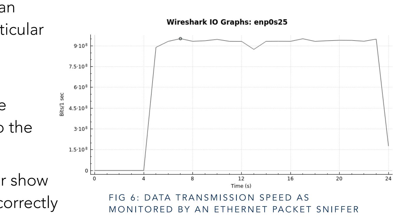
The Ethernet throughput is measured @ ~930Mbps i.e. takes ~18s to send 2GB This is at the limit of the GbE protocol.
