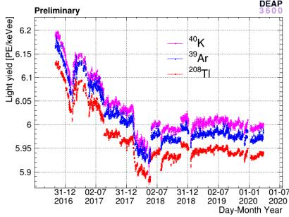
Corrections are applied for the very little variations of light yield for precise measurement of <sup>39</sup>Ar decay events
