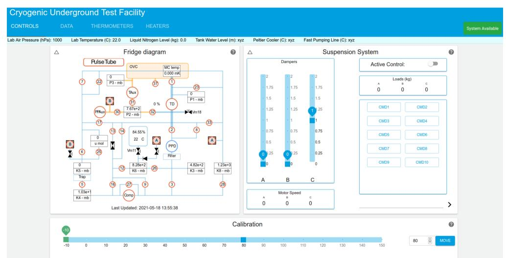
• Slow control system logs environmental parameters collected from sensors around the facility
