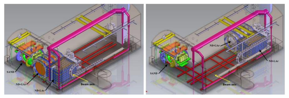
**SAND** System for on-Axis Neutrino Detection = tracker + ECAL  $\Rightarrow$  beam monitor
