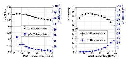
Performance of the  $\pi^+$  identification using calorimeters (left) and RICH (right) measured on 2017 data.
