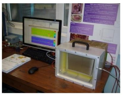
1726 pads Micromegas resistive Kapton bulk
