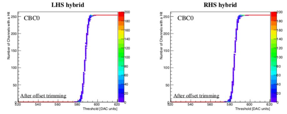
• The difference in the number of hits between every threshold and the next is used characterize the noise per channel :
