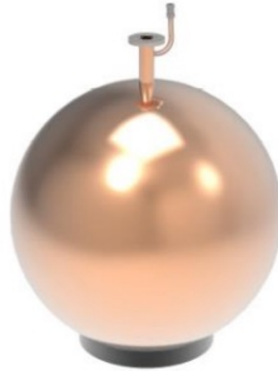
140 cm diameter low activity copper (C10100) SPC 7 - 25 \mu\text{Bq/kg} ^{232}\text{Th} 1 - 5 \mu\text{Bq/kg} ^{238}\text{U} Electropolishing and electroplating
