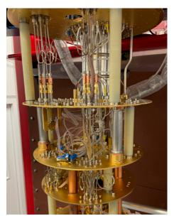
*RF wiring (e.g. for Q-bit work) in a similar facility (NEXUS) at Fermilab*
