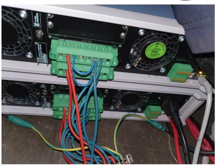
GEM 4 was equipped during the last days of the dry run with two R&S NGP8XX family power supply. Integrated in the DCS system with a readout rate of 10 to 15 Hz. The devices have ben extensively tested in terms of communication stability by Christophe with positive results. Same cabling of GEM0 but interface connector. Network interface (snp)
