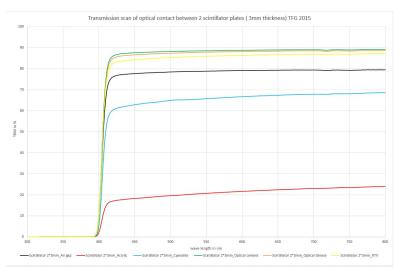
Loctite 406 is suitable for optical gluing of scintillators!
