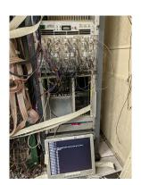
Orsay Discriminator have superior performance in respect to CAEN (double pulse resolution). Infrastructure installed (Modified Crate, CPU, Signal Spliter).
