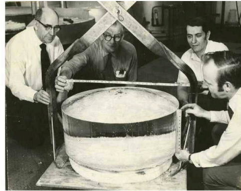
The first 32 inch diameter NaI(Tl) crystal. Pictured from left to right are Dr. Swinehart, Ed Jablon, Joe Knaus and Marko Silgoh.
