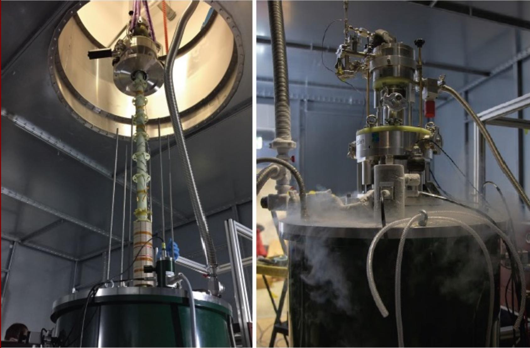
Cryogenics magnet;  $B < 0.15$  T ( $< 1.6$  MHz for  $^{129}\text{Xe}$ )
