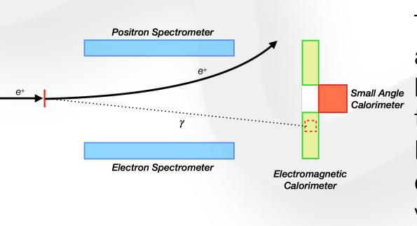
The angular distribution of Bremsstrahlung photons is sharply peaked at small angles to the beam. For this reason, the ECal was built with a Small Angle hole in the centre behind which the Small Angle Calorimeter was built to reject Bremsstrahlung photons.
