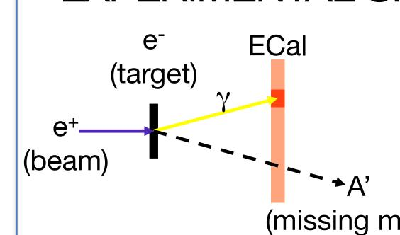
PADME's nominal signal channel looks for the  $\gamma$  produced in associated production with the A'.
