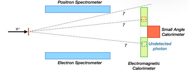
To avoid the loss of annihilation photons, the ECal was built with the highest angular coverage, maximum granularity and best energy resolution possible.
