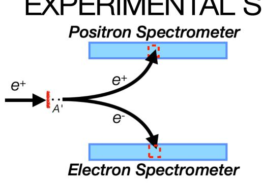
Using the magnetic field and the charged particle spectrometers, we can also search for visible final states.
