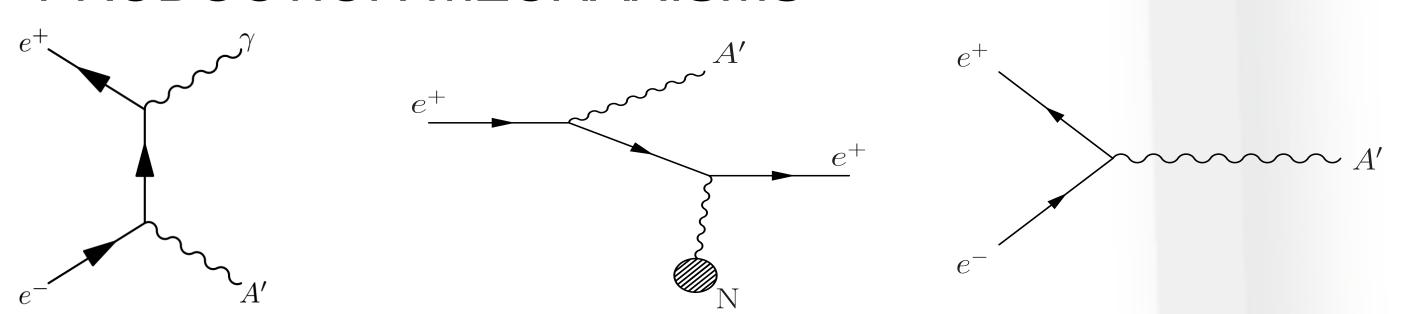
The nominal production mechanism at PADME is associated production of an A' with a SM  $\gamma$  but A'-strahlung and resonant annihilation are also accessible to PADME. All of these mechanisms are identical for both A' and ALPs.
