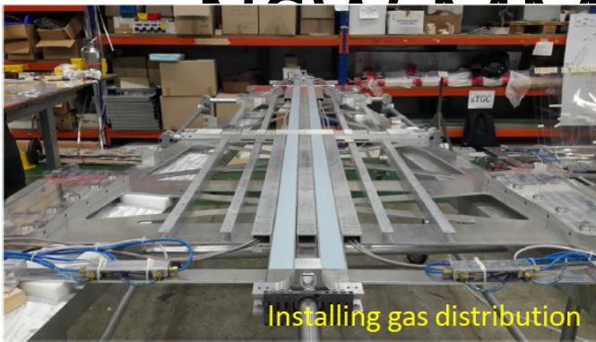
Installing gas distribution on the wedge support
