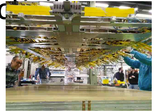
Placing of chamber on the wedge support
