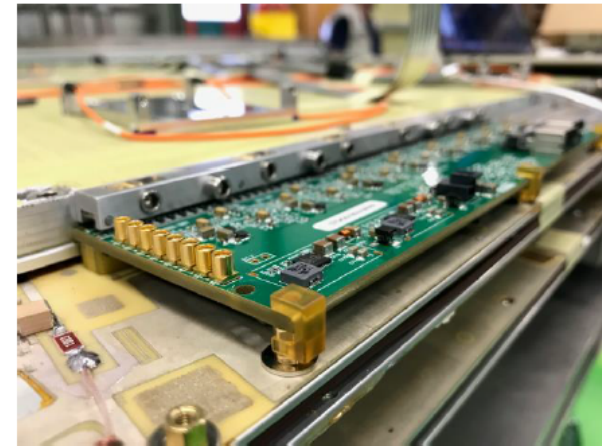
Installing Readout front-end cards
