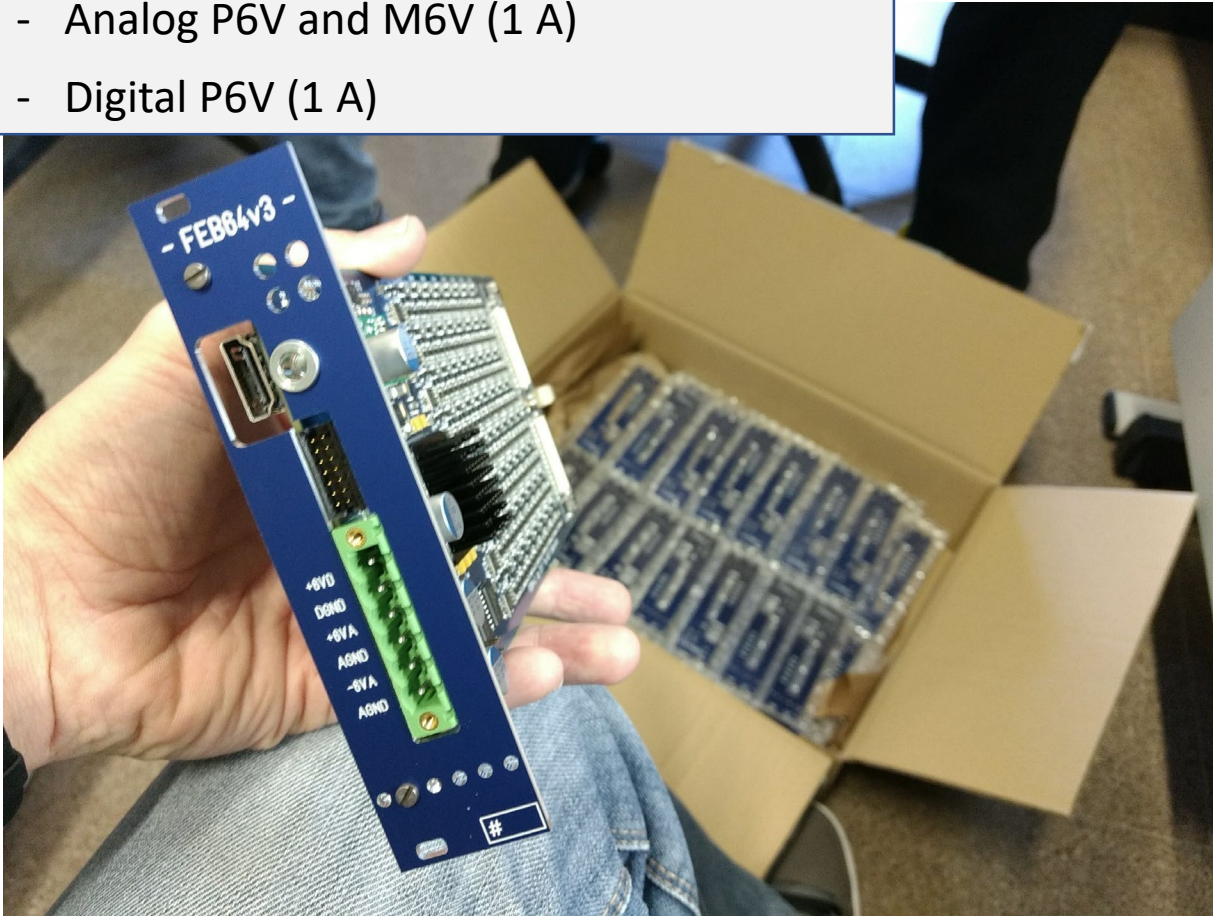
HDMI lock in the FEv3 front panel to avoid disconnections
