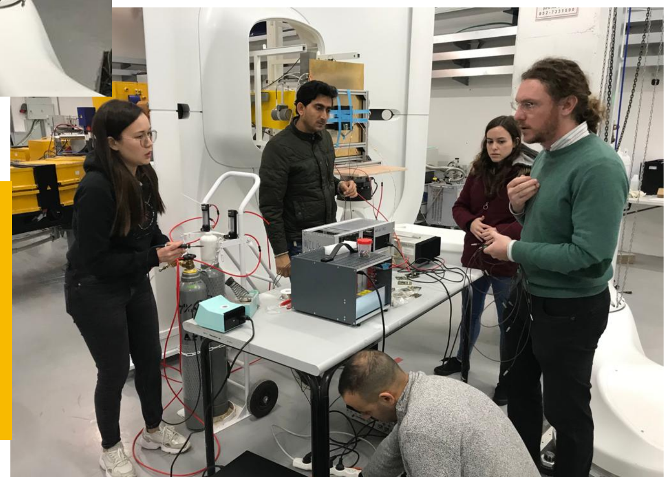
RPWELL setup • Ar/7%CO 2 • HV • readout • scintillators and trigger logic
