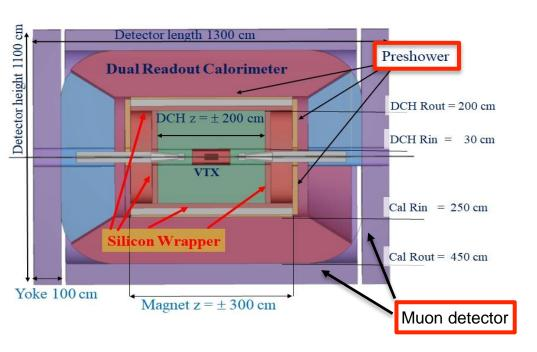
Pre-shower and Muon system based on  $\mu$ -RWELLs technology:
