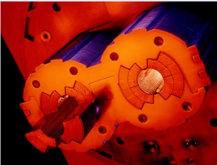
Dipolo normal conductor \rightarrow B_{\max} \sim 1.8 \text{ T}
