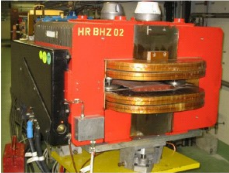
Dipolo normal conductor \rightarrow B_{\max} \sim 1.8 \text{ T}
