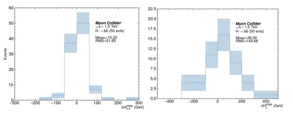
$\Delta H_{miss} = H_{missBIB} - H_{missnoBIB} \rightarrow$  calculated in the transverse and longitudinal plane
