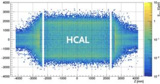
Energy deposition in calorimeters per bunch crossing
