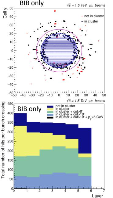
RPC cells of 30x30mm<sup>2</sup> 7 barrel layers, 6 endcap layers Much reduced BIB contribution compared to tracker and calorimeter (~8% of BIB) concentrated in the low-radius endcap region Can be effectively removed with geometrical cut to a level that does not contaminate reconstructed muons
