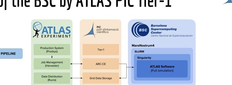
Using two **ARC-CEs** at PIC to interconnect MareNostrum and ATLAS production system
