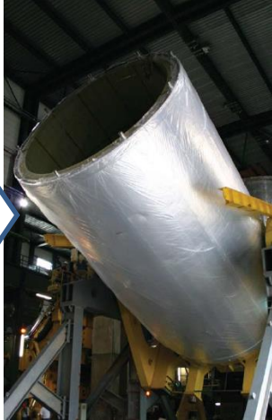
Cold mass rotated 90° and inserted
