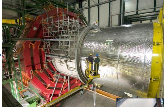
Cold mass rotated 90° and inserted
