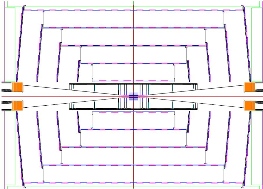
*SiD microstrip tracker: 5 barrels with 4 disks on each side (ILC TDR 2013)*
