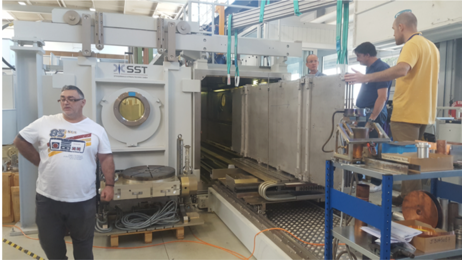
Introduction of the pre-assembled absorber structure inside the EBW machine at CERN
