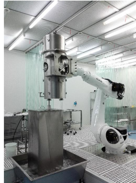
Robot assisting on HPR process
