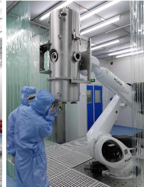
Robot assisting on cavity assembly
