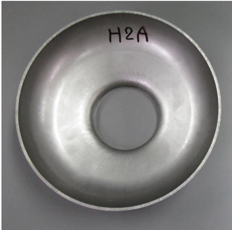
Half-cup: press-formed MG Nb disc.
